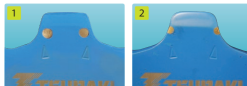
Comparison – New (1) vs. Worn Sprocket (2)
