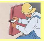
3. Complete installation. After the area has cooled, attach the lever, apply the gasket, and place the safety warning label in a prominent position.
